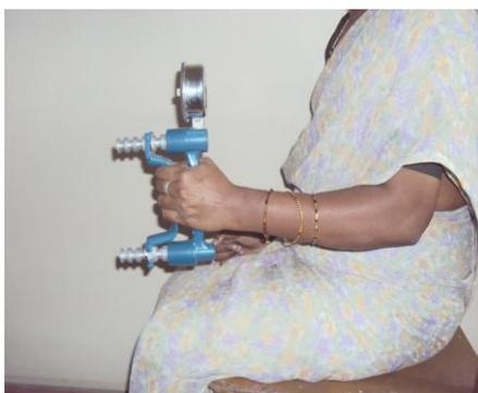
**Fig 1:** Measuring Grip Strength Using Hand Dynamometer
